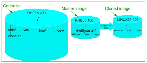
Figure 8-1 Cloning block diagram
