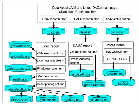
Figure 13-14 DAZL design block diagram
