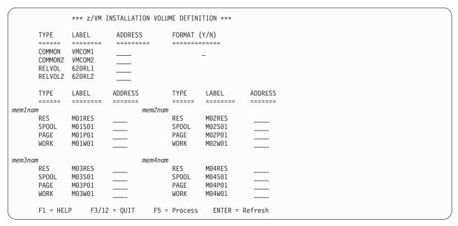
Figure 9. Installation Volume Definition (SSI Only)
