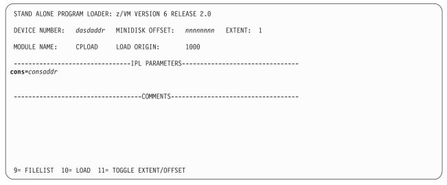
Figure 1. Sample Stand Alone Program Loader Panel
