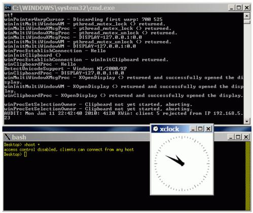
Figure 11-3 Manual setting of DISPLAY variable
