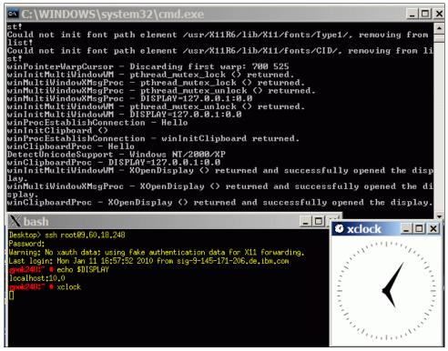
Figure 11-6 X11 forwarding with embedded SSH client
