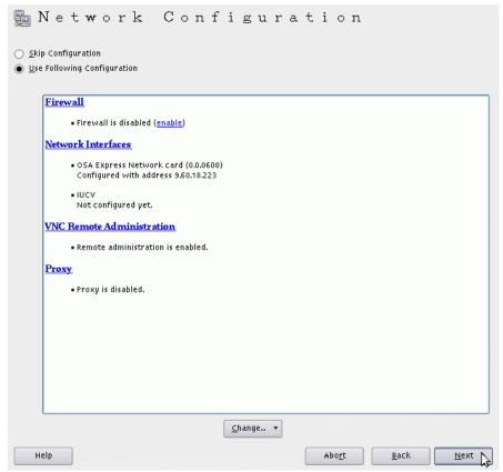
Figure 8-14 Disabling firewall in Network Configuration window
